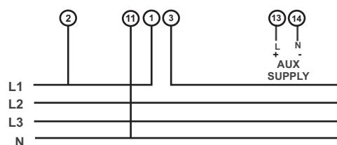
It is recommended that the wires used for connections to the instrument should have lugs soldered at the end. That is, the connections should be made with Lugged wires for secure connections. The Maximum diameter of the lug should be 7.0 mm and maximum thickness 3.5 mm.
