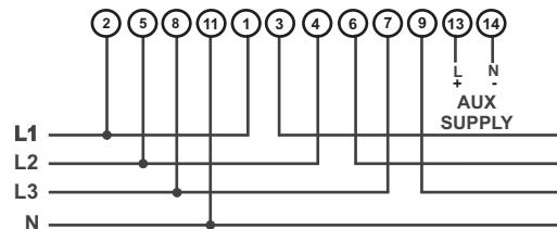
**For 3 Phase 3 Wire Unbalanced Load**
