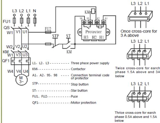
6.2 Wiring diagram for control power supply @ AC22V voltage
